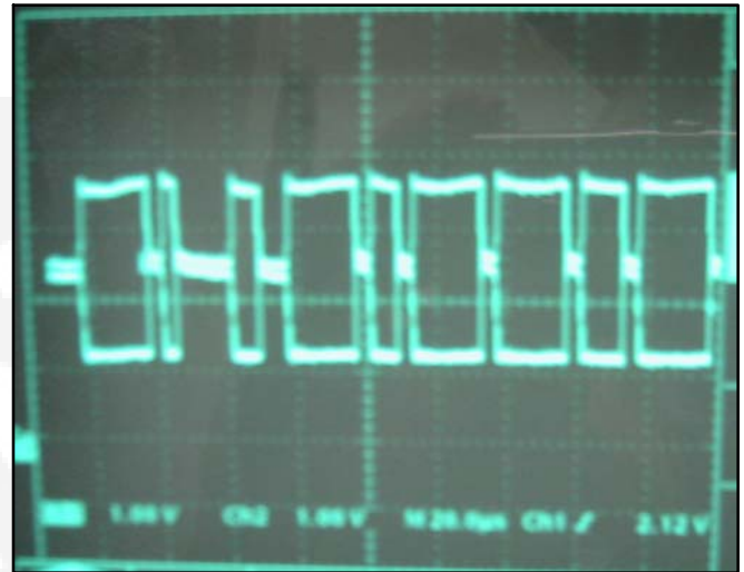
FIGURE 5-7. CAN DATALINK: GOOD SIGNAL
